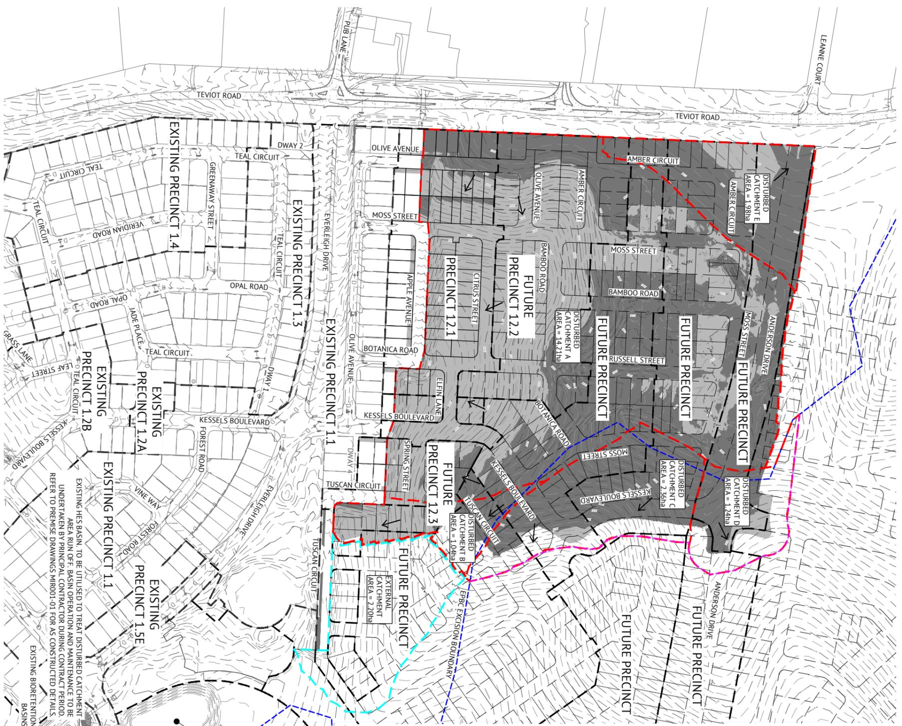
**EXISTING CONSTRUCTION WATER HOLDING DAM. TO BE UTILISED TO TREAT DISTURBED CATCHMENT AREA RUN OFF. BASIN OPERATION AND MAINTENANCE TO BE UNDERTAKEN BY PRINCIPAL CONTRACTOR DURING CONTRACT PERIOD. REFER TO PREMISE DRAWINGS M1R001-01 FOR AS CONSTRUCTED DETAILS.**
